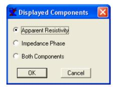
Selecting the pseudosection for MT data allows for display of Apparent Resistivity, Impedance Phase or both.
