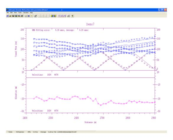
When the iterations are finished, the final result is displayed and the layers are indicated by color on the traveltime vs. distance display. The main point is that the synthetic curves are a good fit to the data curves and the velocities and depths are not too far from the starting values.
