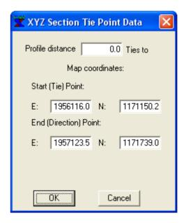
The profile distance must tie to a map point. Here, the map point 1956116.0E, 1171150.2N ties to the beginning of the profile at distance zero.
