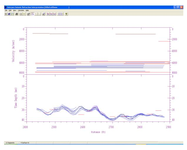
Top graph shows velocities. Surface velocities are the dark lines shown near the top (1000-1250 m/s). The red lines show the velocities determined from time-intercept analysis and the blue and dark blue lines are determined from GRM velocity analysis.
